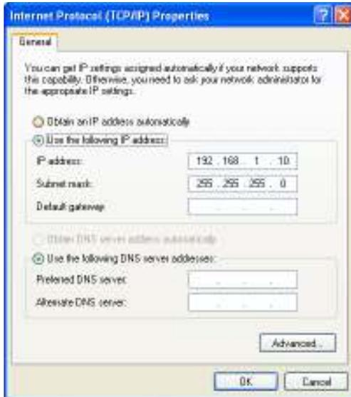
3. Select **Use the following IP Address** radio button and then enter the IP address and subnet mask. Ensure that the IP address and subnet mask are on the same subnet as the device.
