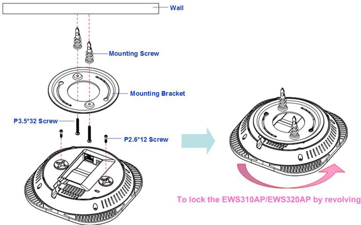
3. Mount the EWS310AP/EWS320AP on the mounting bracket by rotating the unit clockwise about 90 degrees to secure it in place.
