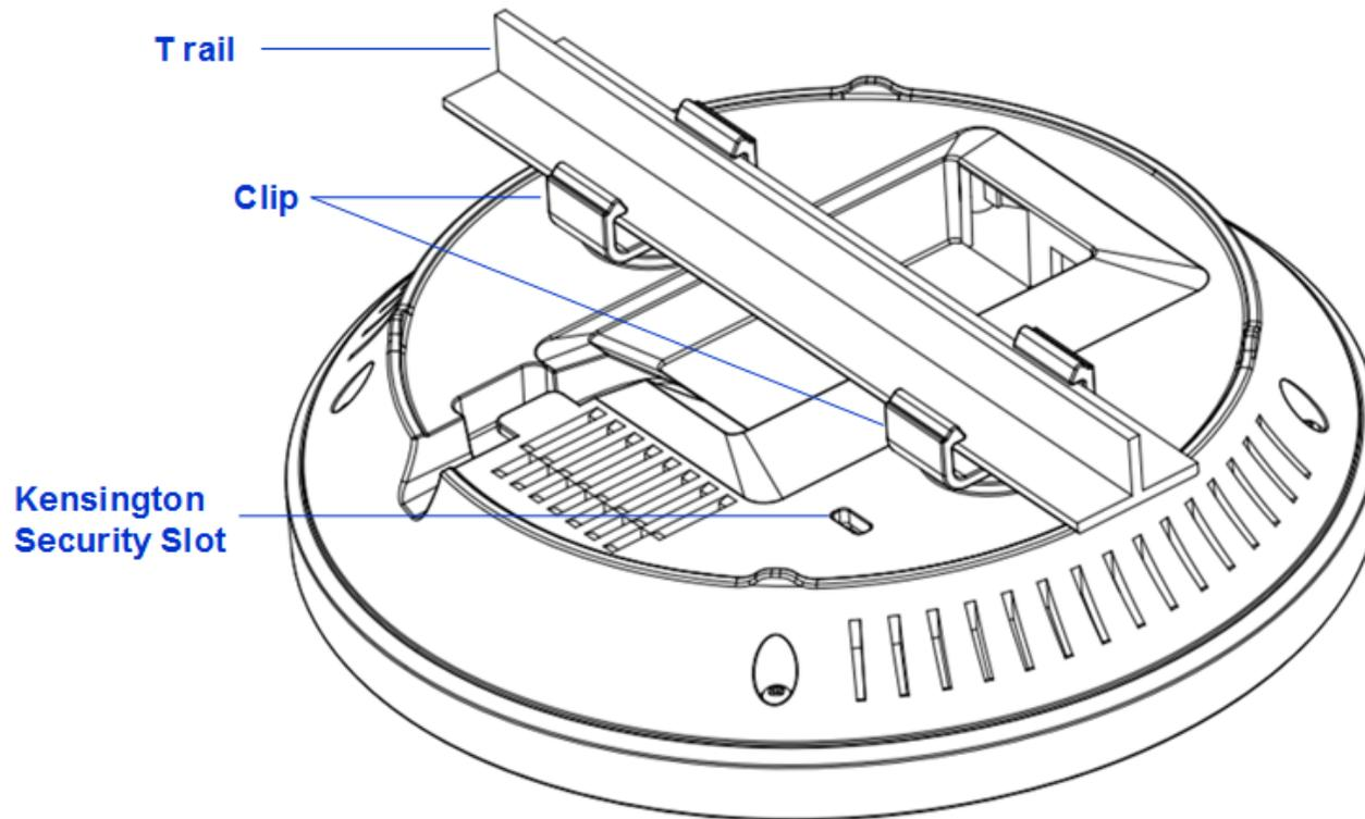
**Note:** To protect your EAP600, use the Kensington security slot to attach a cable lock (cable lock is not included).
