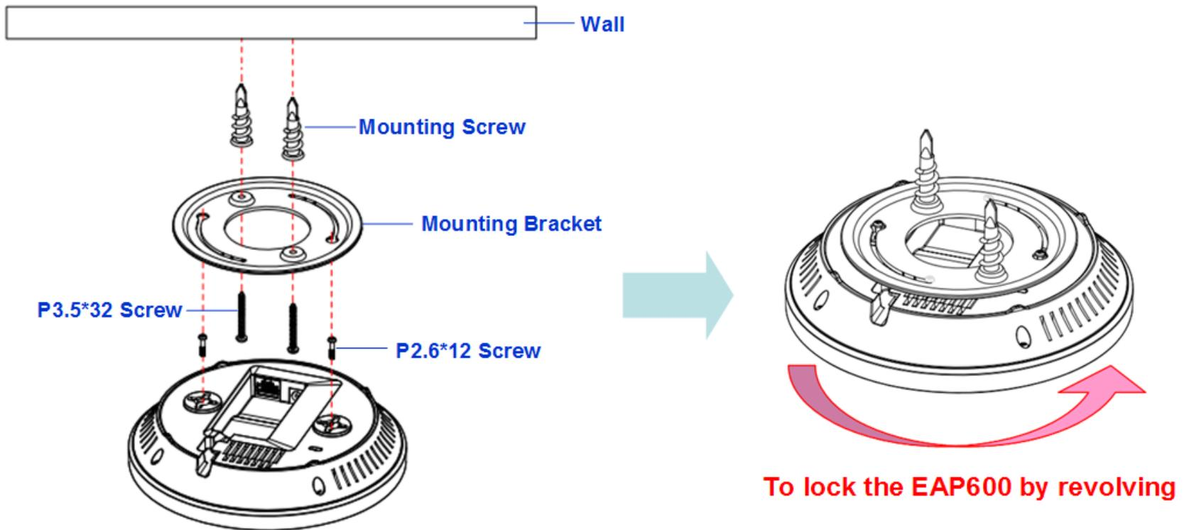
3) Mount the EAP600 on the mounting bracket by rotating the unit clockwise about 90 degrees to secure it in place.
