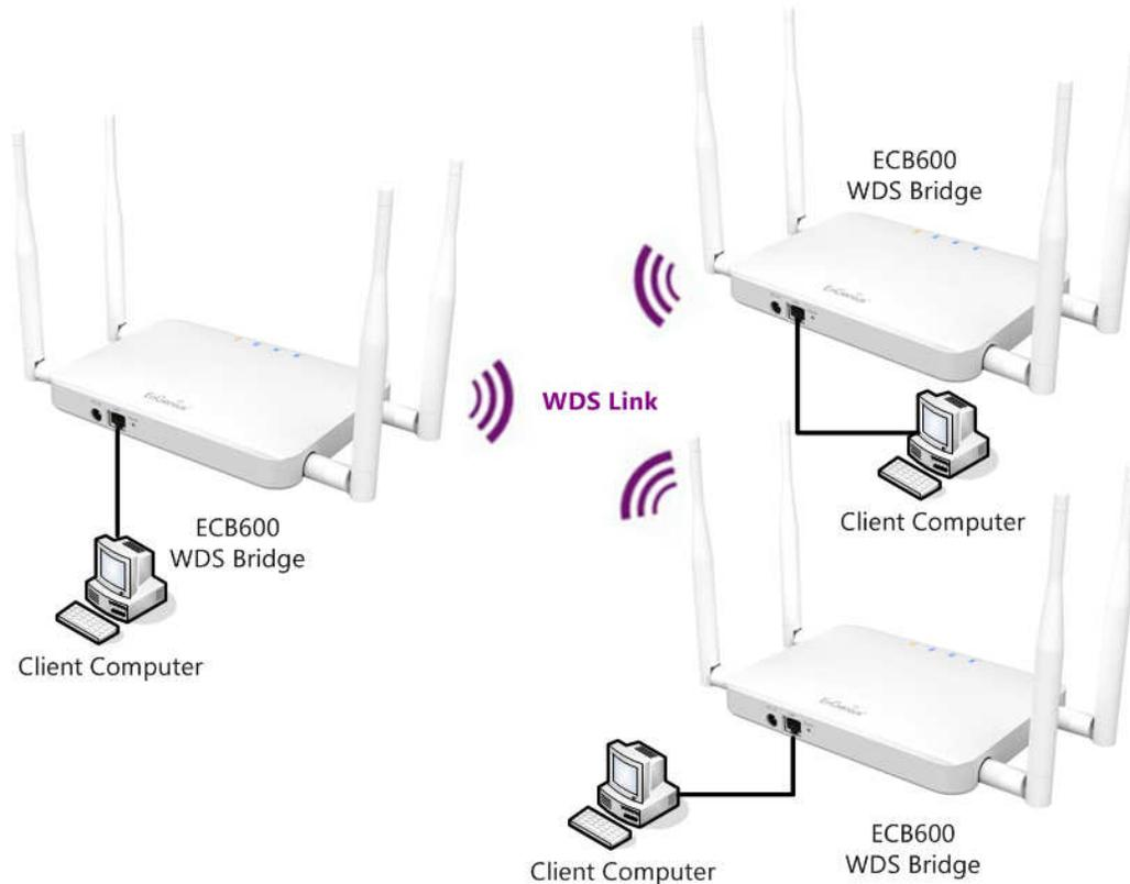
**Note:** WDS Bridge Mode does not act as an Access Point. Access Points linked by WDS are using the same frequency channel. More Access Points connected together may lower throughput. This configuration can be susceptible to generate endless network loops in your network, so it is recommended to enable the Spanning Tree setting (see 6.3 Spanning Tree Setting, below) to prevent this from happening.
