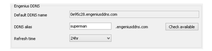
**Default DDNS name**: Each camera has a unique DDNS name printed on the back of your camera. It is the default DDNS name.
