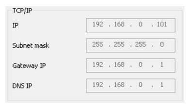
You will need to assign the IP address details in TCP/IP section. Please ensure that the IP address is not being used by someone else in the network.
