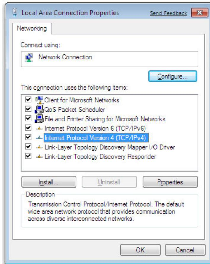
4. In the properties dialog box, click **Use the following IP address:** to configure your computer for Static TCP/IP. Enter an **IP address** (i.e. 192.168.1.10), the **subnet mask** of the ENH202, and the **default gateway** which is the ENH202's IP address, 192.168.1.1. Note: the subnet mask must match that of the ENH202 and the IP address must be on that subnet.
