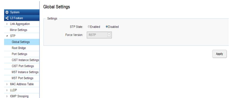
Once a stable network topology has been established, all bridges listen for Hello Bridge Protocol Data Units (BPDUs) transmitted from the Root Bridge of the Spanning Tree. If a bridge does not receive a Hello BPDU after a predefined interval (known as the Maximum Age), the bridge will assume that the link to the Root Bridge is down and unavailable. This bridge then initiates negotiations with other bridges to reconfigure the network to reestablish a valid network topology.
