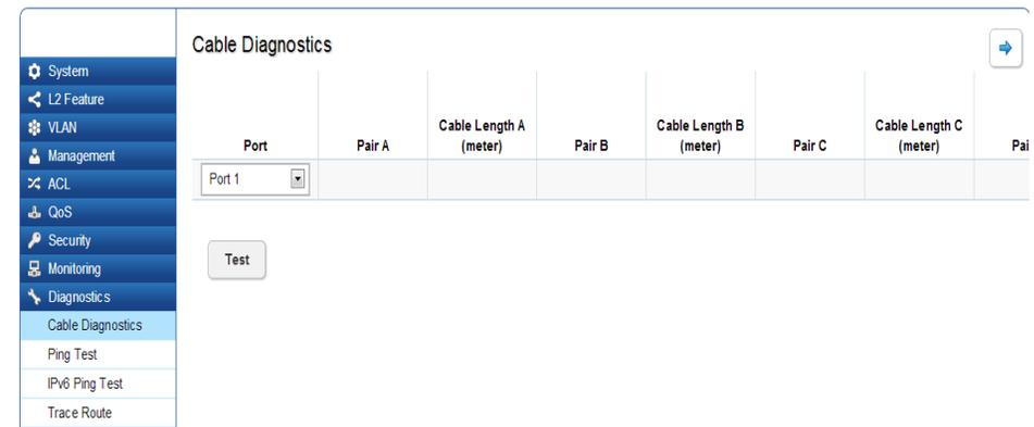
Click **Test** to perform the cable tests for the selected port.
