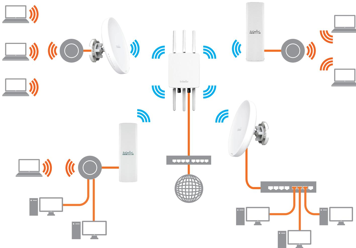
The AP can be used as a centralized Outdoor Access Point with which other EnGenius Wireless 802.11b/g/n 2.4 or ac/a/n 5 GHz Outdoor Client Bridges can associate; leveraging the long-range capability of their internal high-gain directional antennas, resulting in a very cost-effective solution to expand a company network over a multiple building campus.
