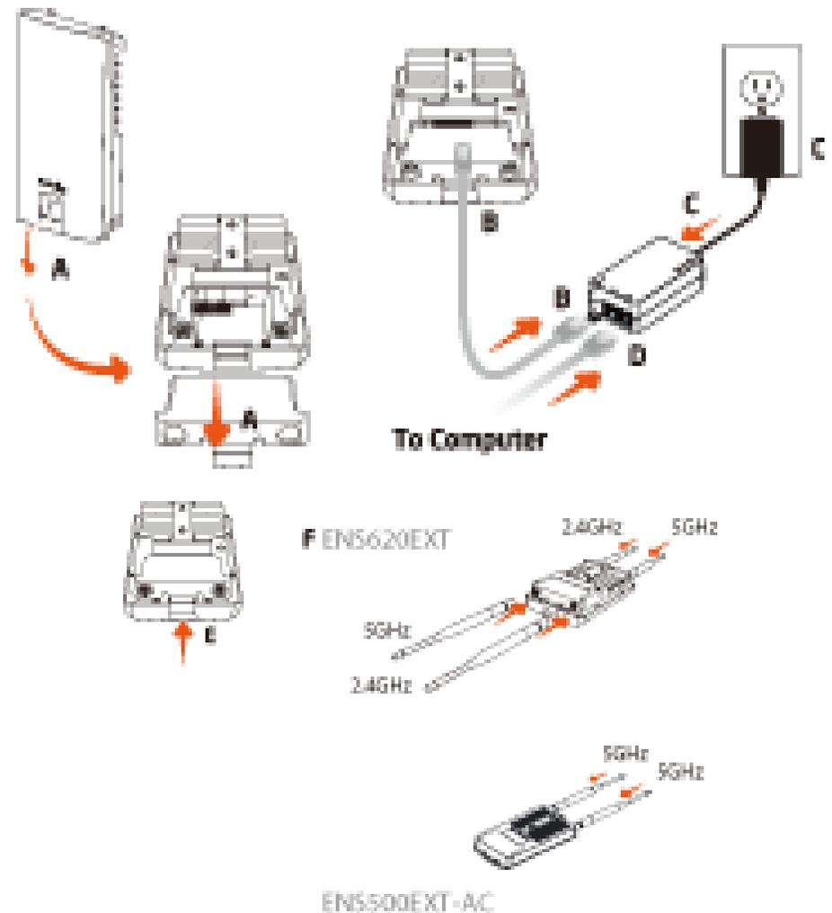
**Note:** The Access Point **NOLY** supports the included proprietary 24V PoE adapter.
