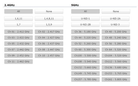
\*Default configuration: Default setting of channel selection is "All" to perform auto channel on the exist channel list.
