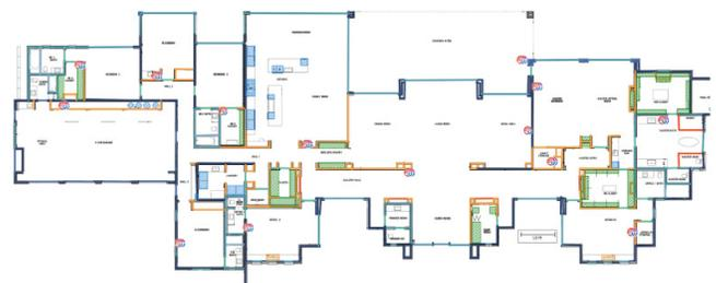
Figure 1: Predicted AP Placement [Ground Floor]
