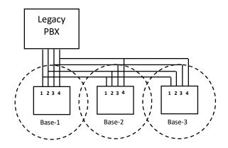
Re: when a call is coming in from L1, all handsets can pick up the call, as long as the handsets are in the coverage of base1~3.
