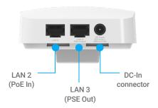
\*Only one port of LAN 1/ LAN 2 can be chosen for PoE-In mode simultaneously
